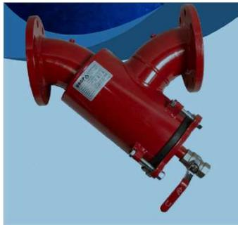
Strainer filters - SY series are used to protect irrigation network equipment (such as pumps, valves, etc.) from wear and blockage by the presence of large caliber sediment. All filters are PN16 and the product range can serve large number of flow. The installation of the filter is done by following the direction of the flow arrow in the filter body.
